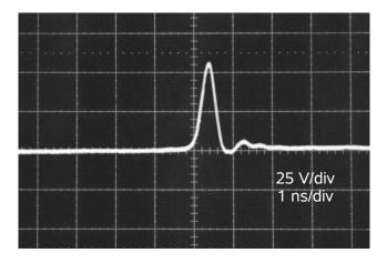
The AVMH family of low jitter, high amplitude impulse generators includes units providing pulse widths in the range of 200 ps to 1 ns, amplitudes from 10 Volts to 100 Volts, and pulse repetition frequencies as high as 20 MHz.
